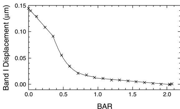
**Fig. 4.** The displacement in the Band I center in olivine-orthopyroxene mixtures relative to the Band I center for the pyroxene phase as a function of the band area ratio (BAR). BAR is inversely proportional to olivine abundance.
