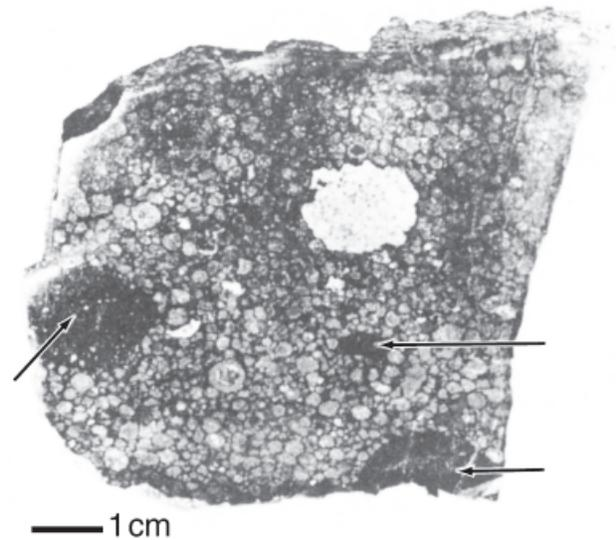
**Fig. 1.** Polished slab of the Leoville CV3 chondrite showing numerous chondrules, one large and several small, white Ca-Al-rich inclusions (CAIs), and three dark inclusions, which are marked by arrows. Chondrules and CAIs formed in the solar nebula but dark inclusions are probably fragments of preexisting bodies that accreted with chondrules and CAIs. (Photo courtesy of Alfred Kracher and Klaus Keil.)
