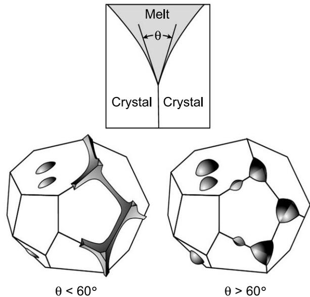
**Fig. 1.** Illustration of the dihedral angle  $\theta$  and a depiction of two endmember microstructures for static systems. At  $\theta < 60^\circ$ , an interconnected network will form and melt migration can occur. If  $\theta > 60^\circ$ , melt forms isolated pockets. In experimental systems, interconnectedness occurs in static systems only if they are anion-rich.
