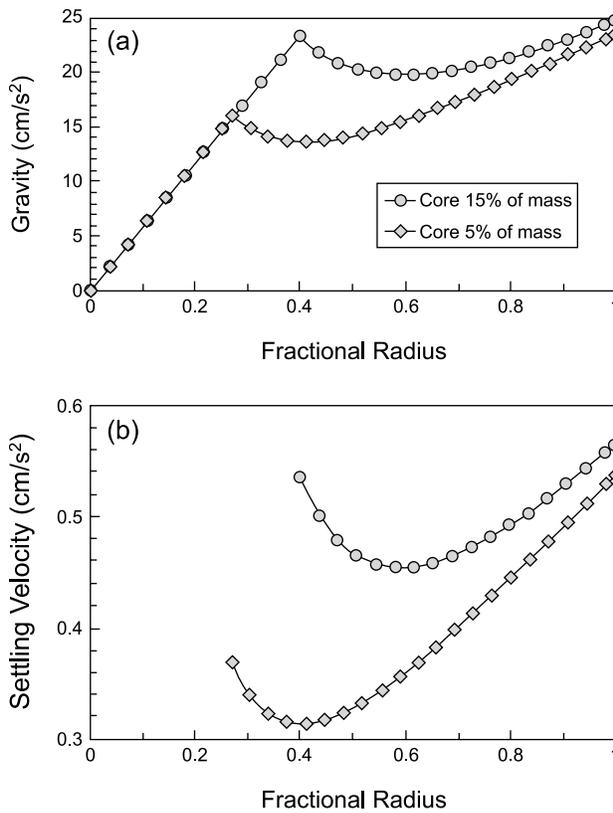
**Fig. 6.** Calculated (a) gravity and (b) grain-settling velocity vs. fractional radius for a Vesta-sized molten asteroid. Core density calculated for a mixture of 90% Fe,Ni and 10% FeS; silicate melt density is  $2900 \text{ kg m}^{-3}$ , following *Richter and Drake* (1997). Settling velocity calculated following *Walker et al.* (1978) assuming 1-cm grains with a density of  $3200 \text{ kg m}^{-3}$ .
