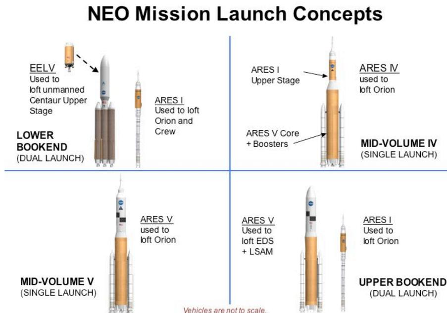
**Figure 1:** The four types of NEO mission launch concepts considered for the Constellation NEO feasibility study.
