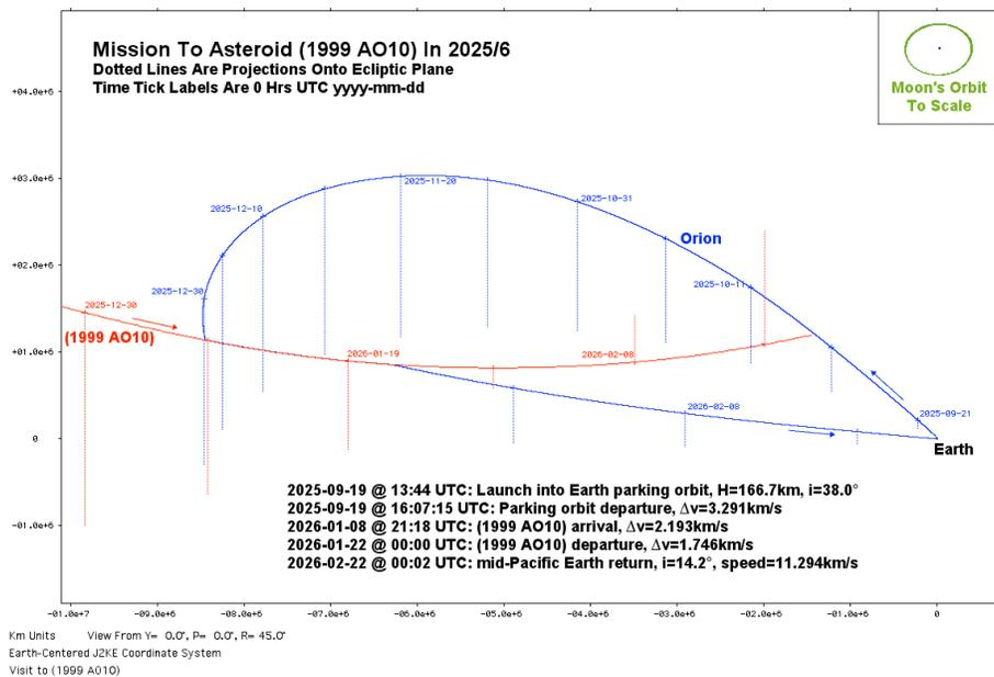
**Figure 2:** An Earth-centered trajectory plot showing a possible 150-day mission profile to NEO 1999 AO<sub>10</sub> with the CEV on top of an Ares V launch vehicle. Atmospheric re-entry is similar to that of the Apollo missions returning from the Moon. The Moon's orbit is shown for scale.
