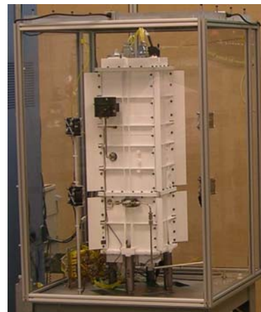
Figure 4: Advanced Stirling Radioisotope Generator (ASRG) and Engineering Unit.
