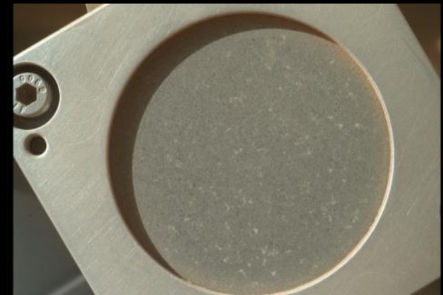
BT2 –basalt from NM, APXS Calibration target, cut and polished in Northrop Hall
