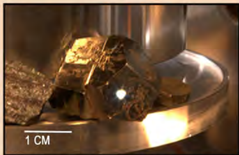
LIBS spark on a piece of iron pyrite. [1]
