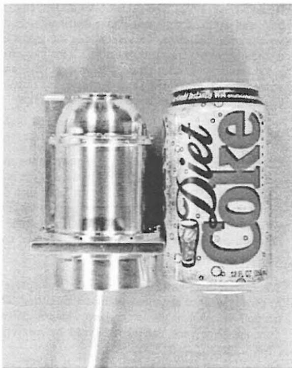
Figure 1 - The FIPS entrance system is compact and lightweight, comparable to a soft drink can in size
