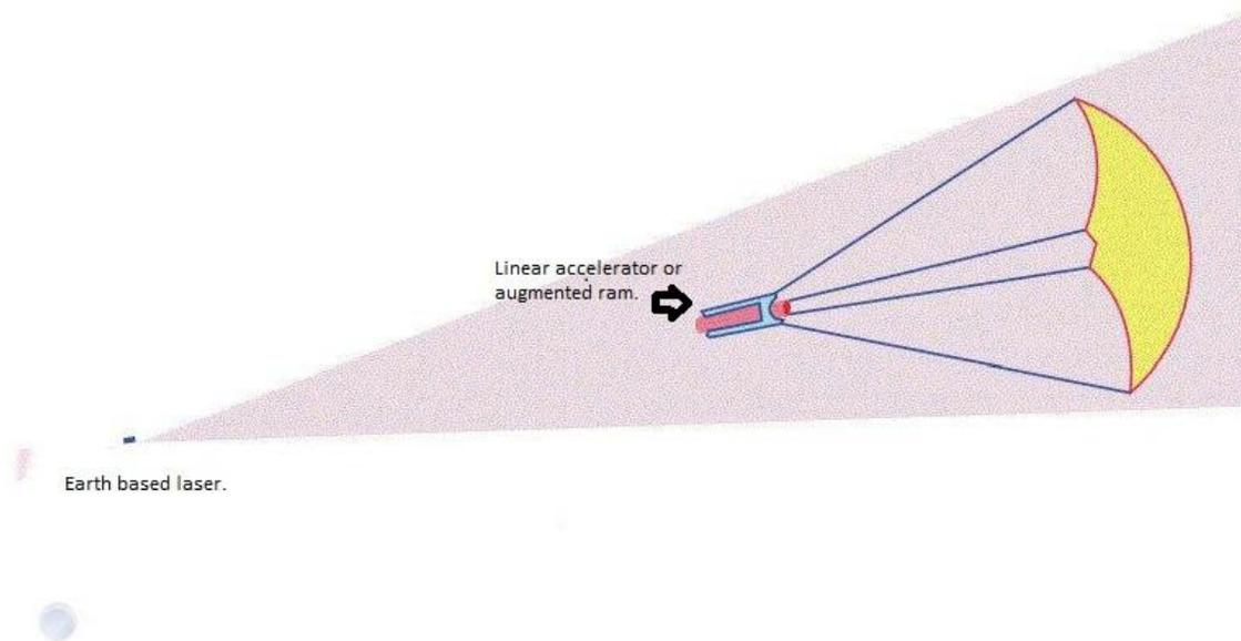
Figure 3. Schematic of Laser Powered or Augmented Ramjet.
