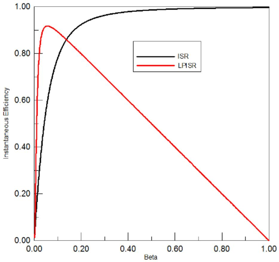
Figure 5: Ramjet efficiency vs beta = v/c.
