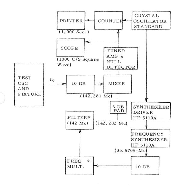
NOTE: The Test Fixture and unit under test must be enclosed in a temperature shield when short-term stability measurements are to be recorded.
