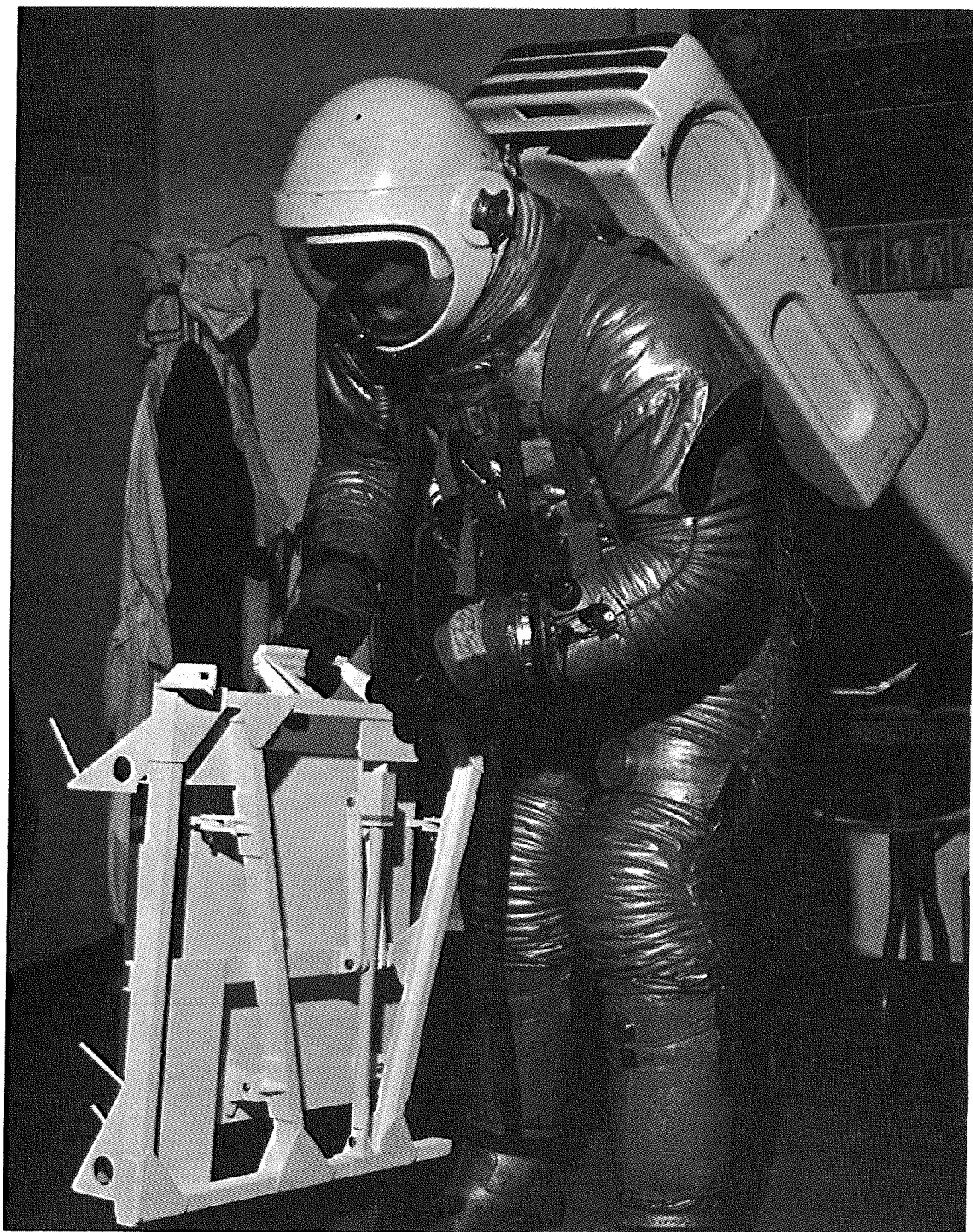
Figure 4 — Test Subject Removes Leveling Leg Pull Pin
