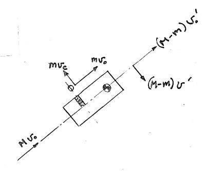
Figure la. Diagram showing ejection of slide and momentum before and after the event
