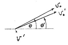
Figure 1b. Vector Diagram of velocities after the ejection of the slide
