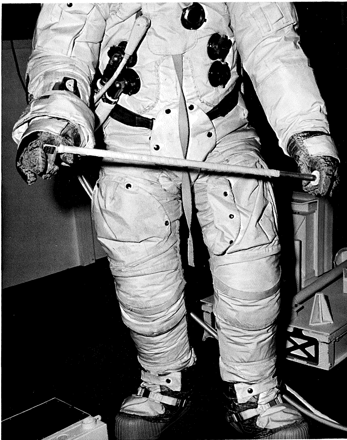
Picture No. 4 Breakseal Removal from UHT
