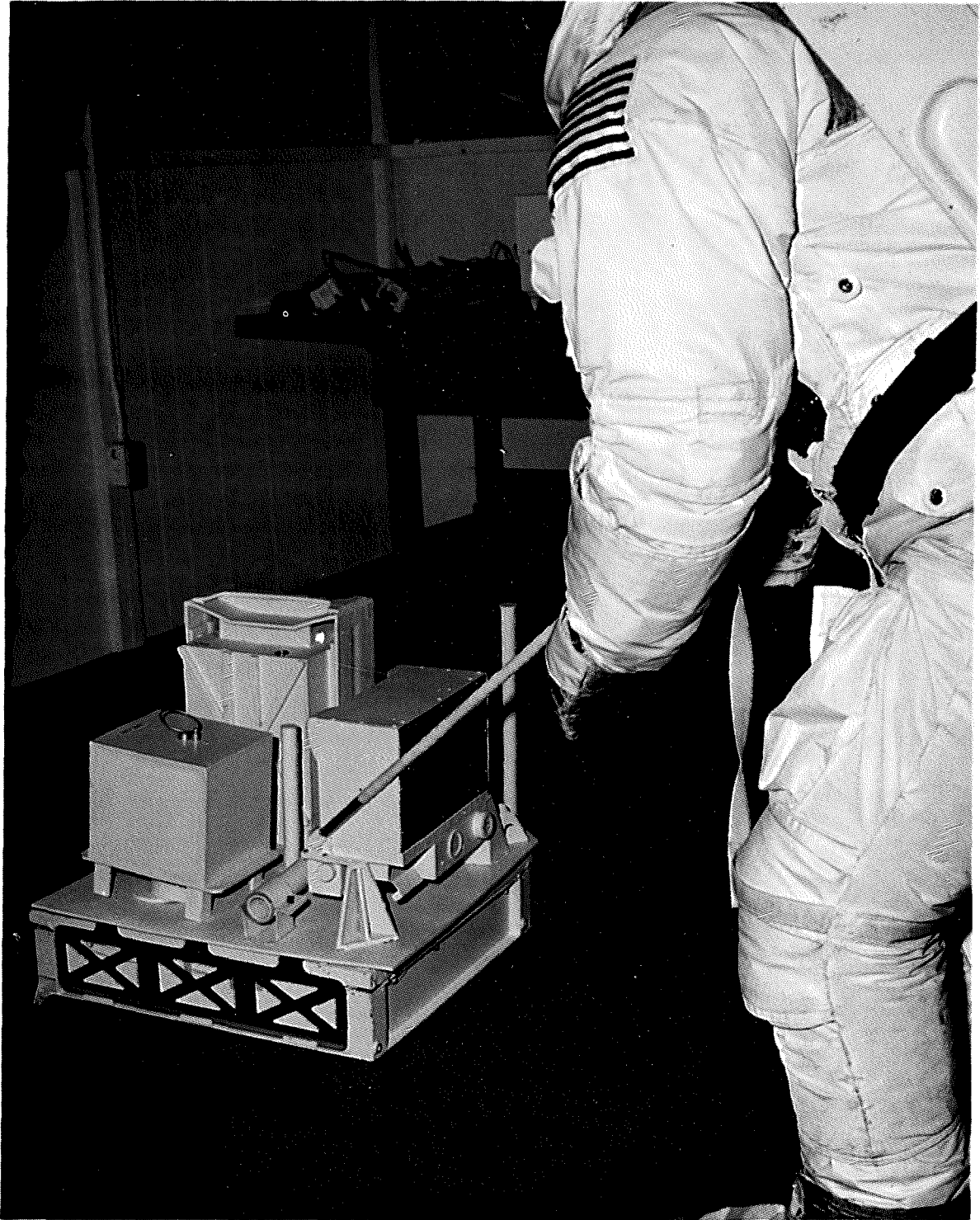
Picture No. 1 LMS Mounted on SP #1 Mockup - UHT Engagement in LMS Carry Socket
