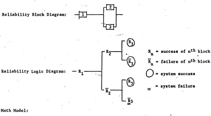
FORMAT 1  $R = R_1 R_2 R_3 + R_1 R_2 \overline{R}_3 + R_1 \overline{R}_2 R_3$   $= R_1 R_2 [R_3 + \overline{R}_3] + R_1 \overline{R}_2 R_3$   $= R_1 [R_2 + (1 - R_2) R_3]$  = [.99974] [.95661 + .04339 (.95894)]= .99795
