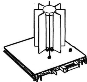
RTG is placed 9 to 12 ft. from and ±20° East or West of Central Station as visually determined by astronaut to minimize thermal load on Central Station.
