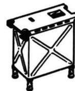
The CPLEE is deployed 9 to 10 ft. North of the Central Station. Bottom of experiment should not touch the lunar surface. It must be leveled to within 2.5° of vertical using bubble level. It must be aligned to within ±2° of East-West sun line. Astronaut will align so that arrow on top of unit points East, then report, within ±1°, the reading of the shadow of the handling tool on the partial compass rose.
