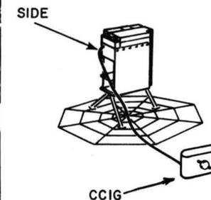
The SIDE incorporates a Cold Cathode Ion Gauge (CCIG). The experiments are deployed 55 ft. SE, SIDE on a ground screen within 5° of vertical, ±5° of E using bubble level and UHT shadow, detectors away from subearth point.
