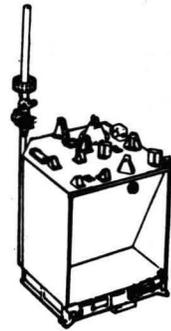
The Central Station is deployed due West or East of LM, preferably West. It must not be deployed in shadow of LM. It is leveled to 5° of vertical as noted by astronaut on bubble level. It is aligned to ±5° of East-West by astronaut using partial compass rose. Closed or curtained sides of Central Station must face East-West.
