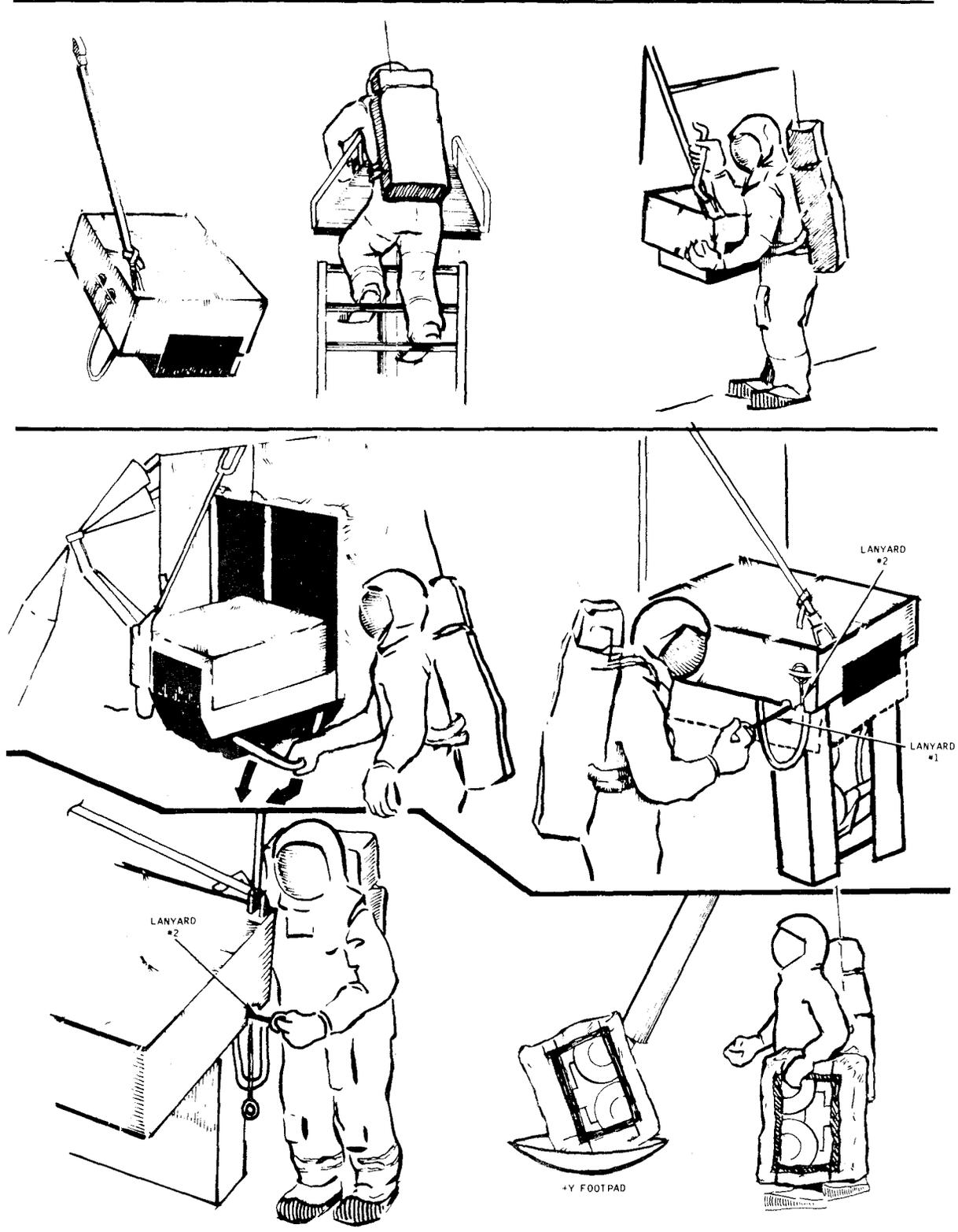
Equipment Transfer Bag (ETB) from the SRC table (the ETB is stowed under the SRC table at launch). This bag has two extra weigh bags and a 100-ft safety tether stowed in it. These items are interim stowed on the MESA for later use. Their place is taken by two Lithium Hydroxide (LiOH) canisters, which are PLSS expendables for use of EVA 2.
