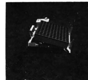
The LR<sup>3</sup> is a deployable array of 100 quartz reflectors aligned by astronaut to reflect laser beams aimed from earth. Pallet is deployed 100 ft W of ALSEP, bubble-leveled and gnomon aligned to 3°, then array is positioned to preset angle. This experiment is completely passive.
