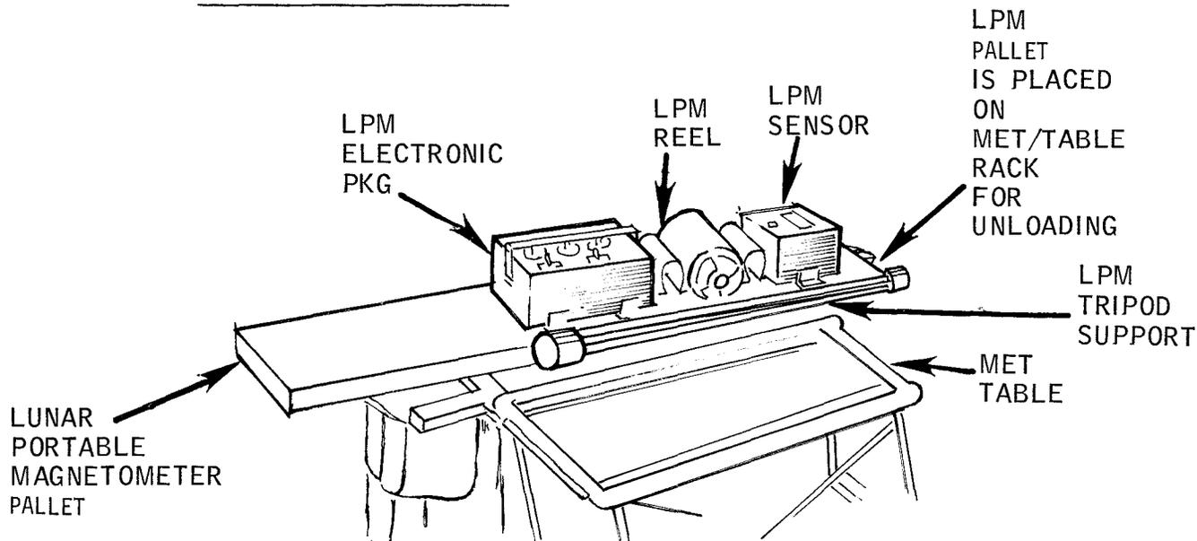
DEPLOYED AND READY FOR USE - 250 OR MORE FEET FROM LM FOR POINT MEASUREMENT
