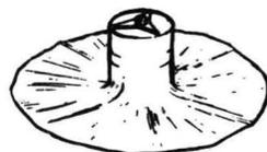
The PSE is deployed 8 to 9 ft. from and Northwest of Central Station as visually determined by astronaut. It must be out of field-of-view of Central Station radiator. It is leveled to 5° of vertical as noted by astronaut on bubble level. Initial alignment is to ±20° of East, before opening PSE shroud. Final alignment will be reported after thermal shroud deployment. The astronaut will give gnomon shadow reading on compass rose, to allow known PSE alignment to 5° accuracy.
