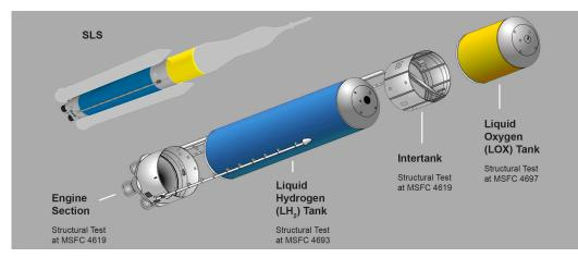
An expanded view of the core stage for NASA's Space Launch System, shows the position of the liquid oxygen and liquid hydrogen tanks that will be tested in the new structural test stands 4693 and 4697 at Marshall.
