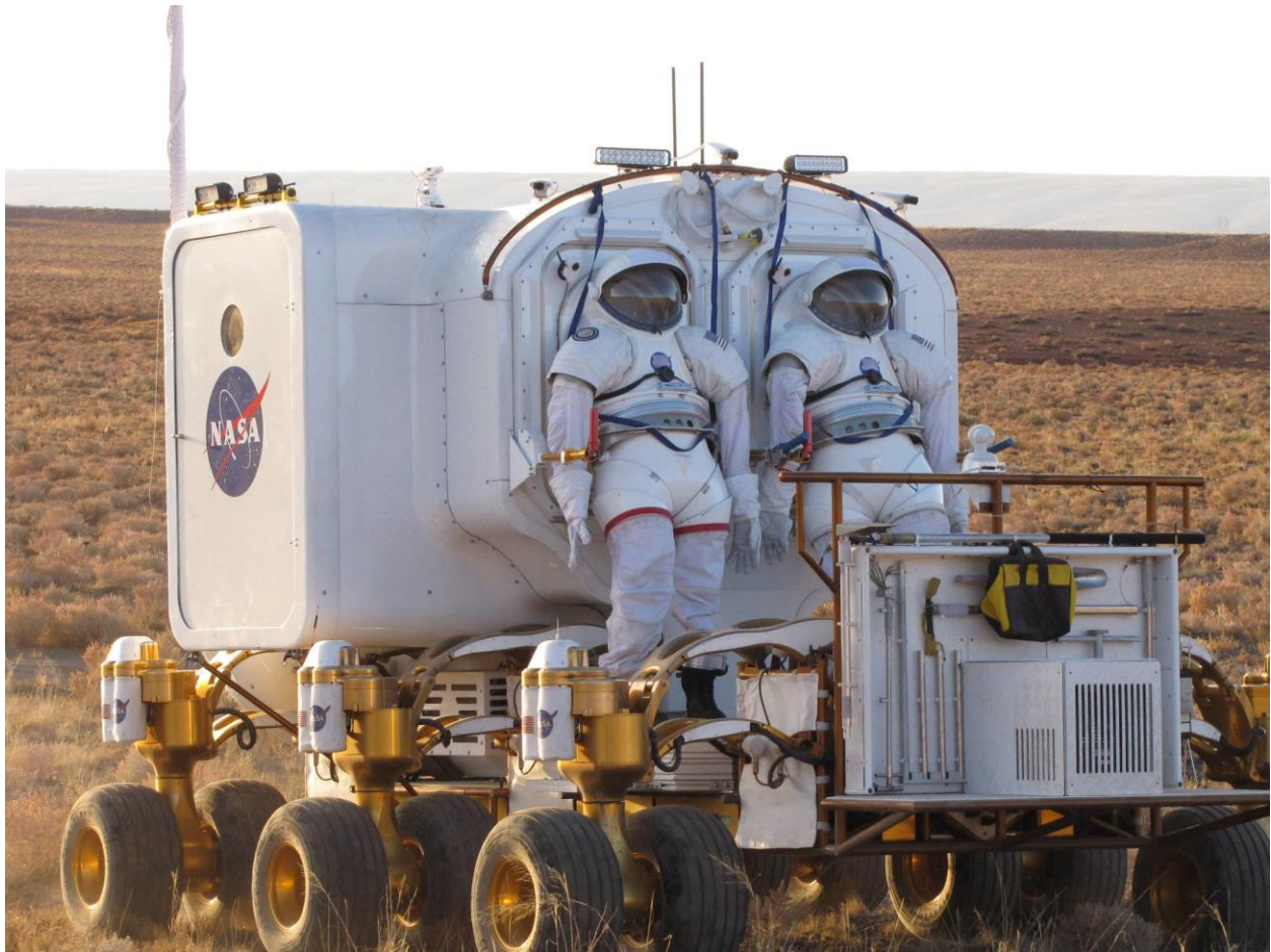
Fig 1: Earth version of the Lunar Electric Rover, created for technology development
