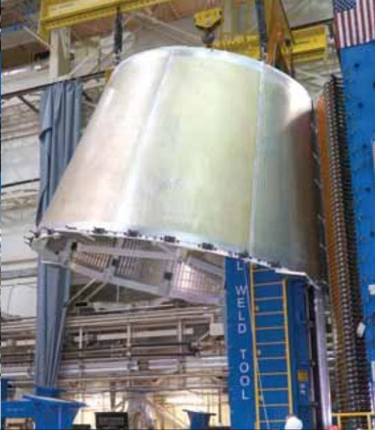
**SLS LAUNCH VEHICLE STAGE ADAPTER CONE**
