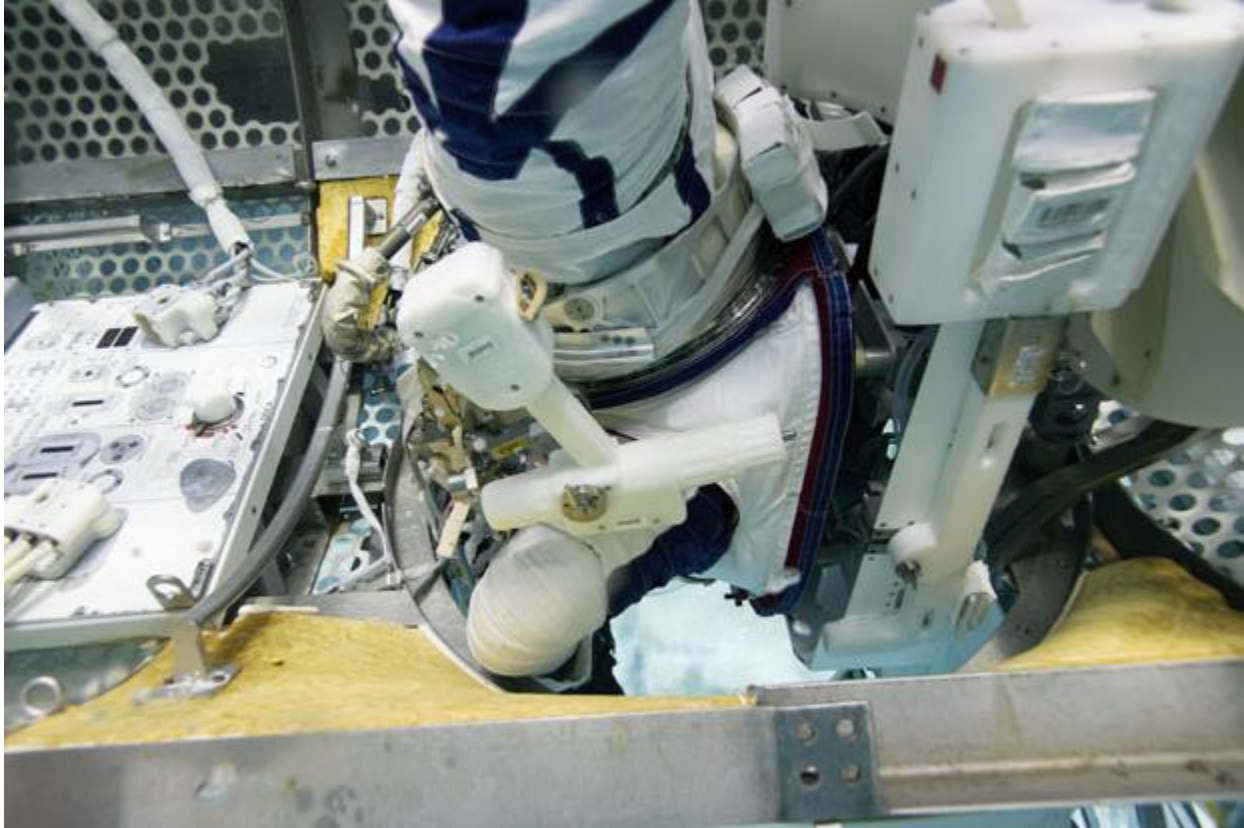
Figure 4: Limited clearances for airlock ingress/egress due to Z-2 system depth
