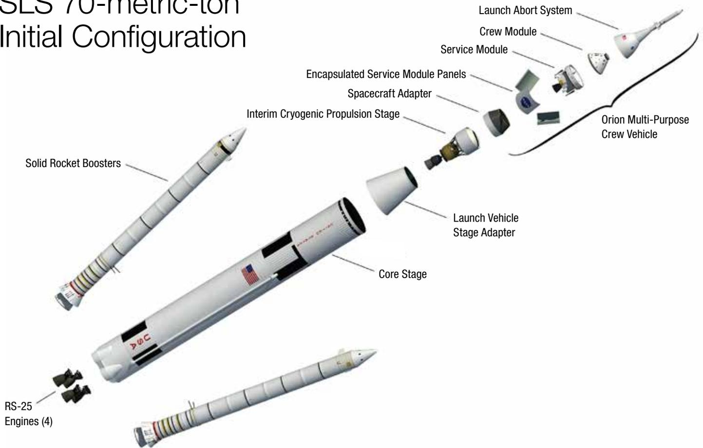
Providing an evolvable architecture allows customization of the SLS to fit individual mission requirements, increasing capability with each configuration.
