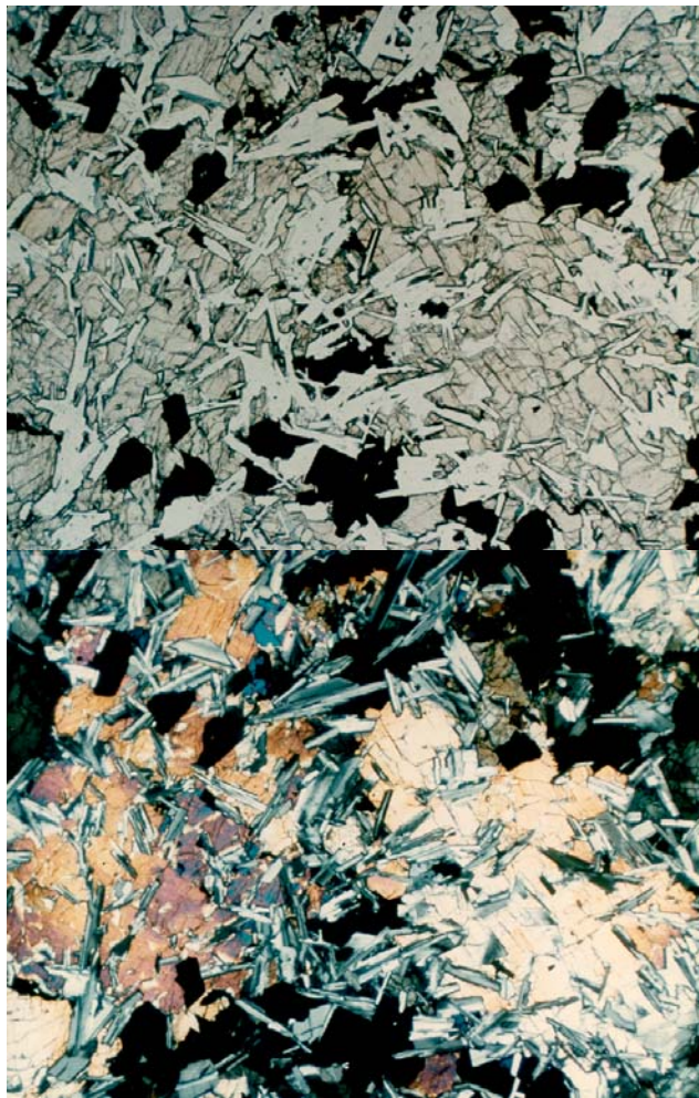
Figure 2: Photomicrographs of thin section 10003,37 (plane polarized and crossed polarized). Width is 2.6 mm. NASA S70-49473-49474.
