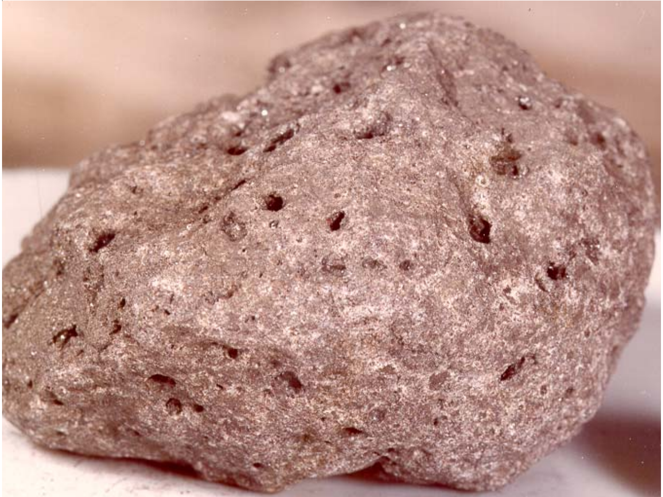
Figure 1: Photo of 10045,19 showing large vesicles and small micrometeorite craters on rounded surface. Scale about 4 cm. NASA S75-31805.
