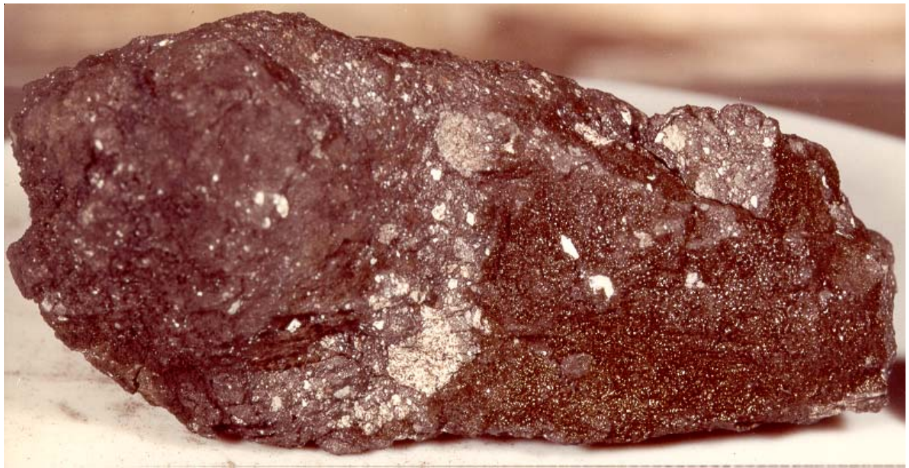
Figure 6: Photo of 10056,14 showing frothy side. NASA S75-32572. Sample is 7 cm.
