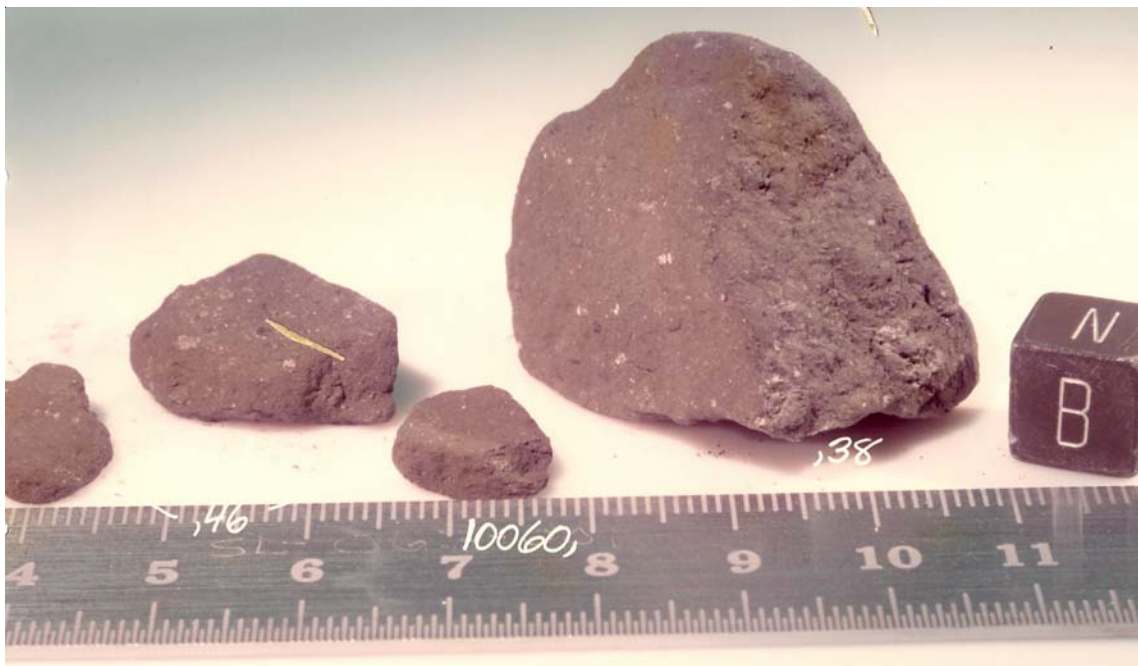
Figure 9: Photo of 10060,38 showing saw cut. Cube is 1 cm. S76-25549.
