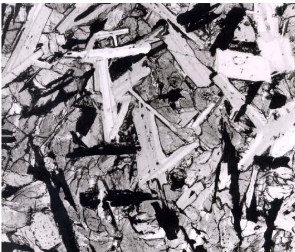
Figure 2: Photomicrograph of thin section of 10062 showing ophitic texture. Field of view about 2 mm. NASA S76-26268.
