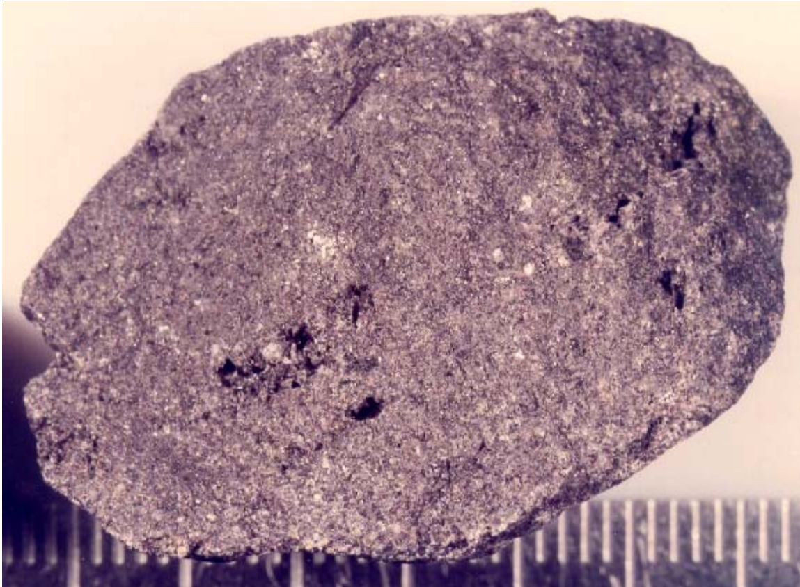
Figure 1: Closeup photo of 10062,13 showing vugs in ilmenite basalt. This is the largest remaining piece (25g). NASA#S76-21515. Scale in mm.
