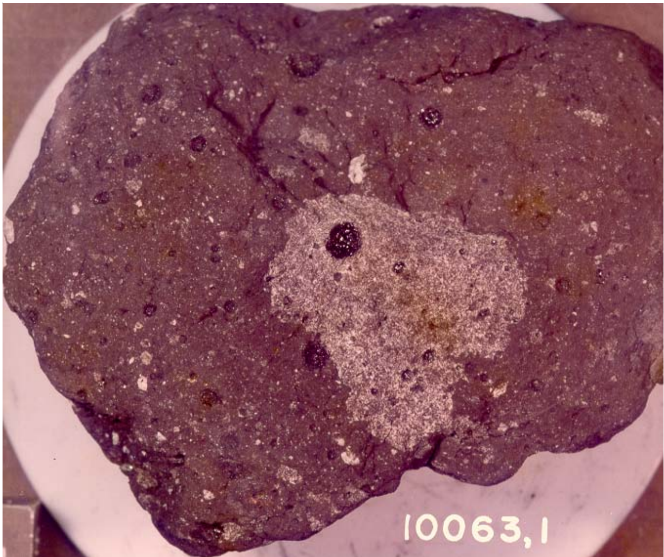
Figure 2: Photo of bottom of 10063,1 showing large (2 cm) clast of basalt (with large zap pit). NASA S75-30489.
