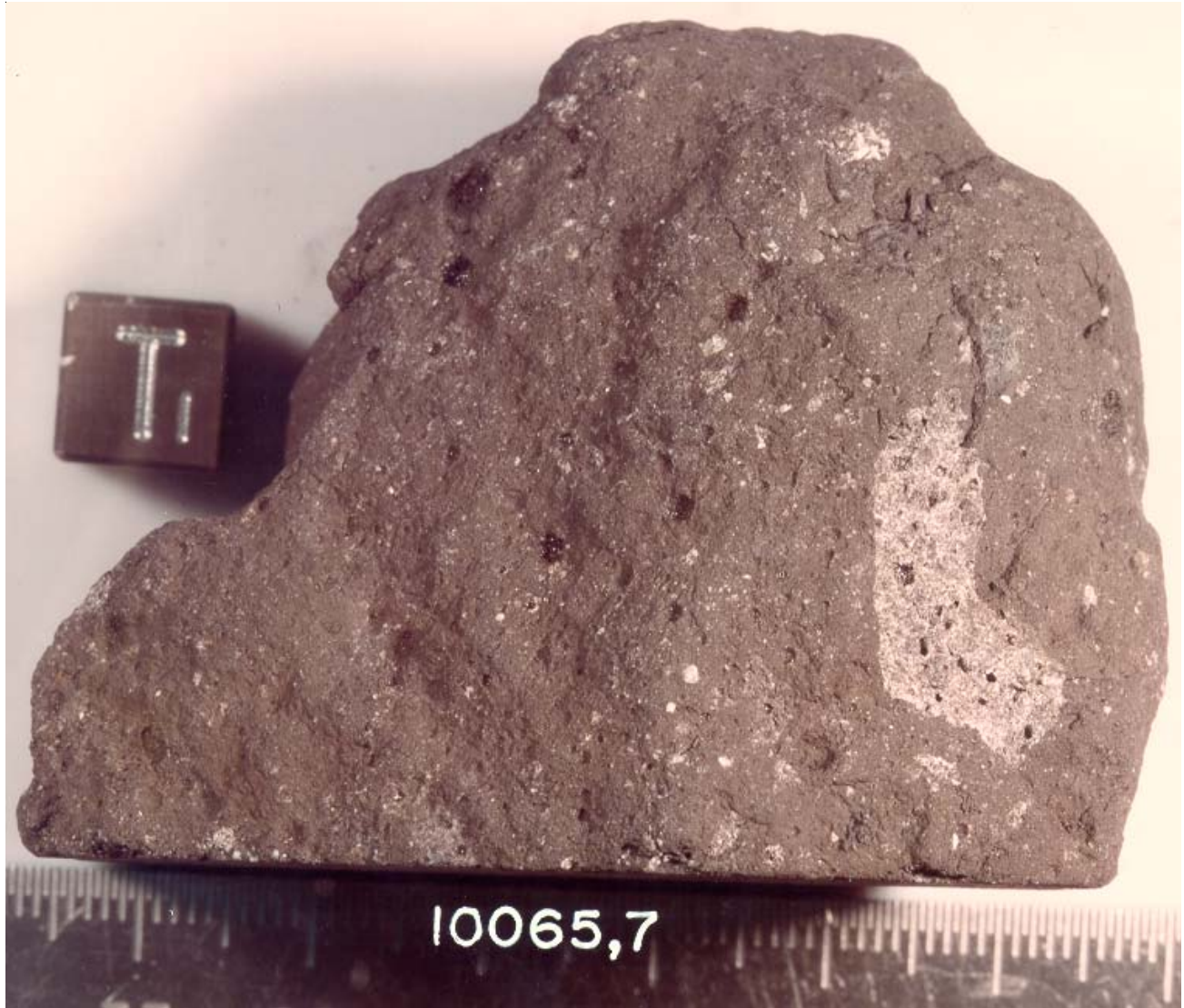
Figure 1: Butt end of lunar breccia 10065,7. Sample is 6 cm across. Cube is 1 cm. NASA S76-22547.
