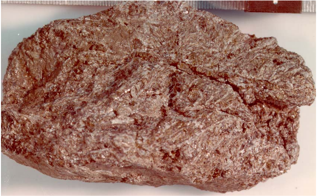
Figure 1: Freshly-broken, hackly surface of 12007 showing elongate pyroxene crystal. NASA photo# S76-25877. Edge of cube at top is 1 cm.
