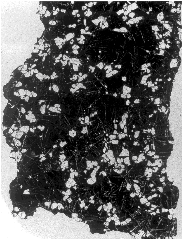
Figure 2: Photomicrograph of thin section 12008,20 showing olivine phenocrysts in nearly opaque groundmass. NASA # S76-29979. Length about 3 mm.
