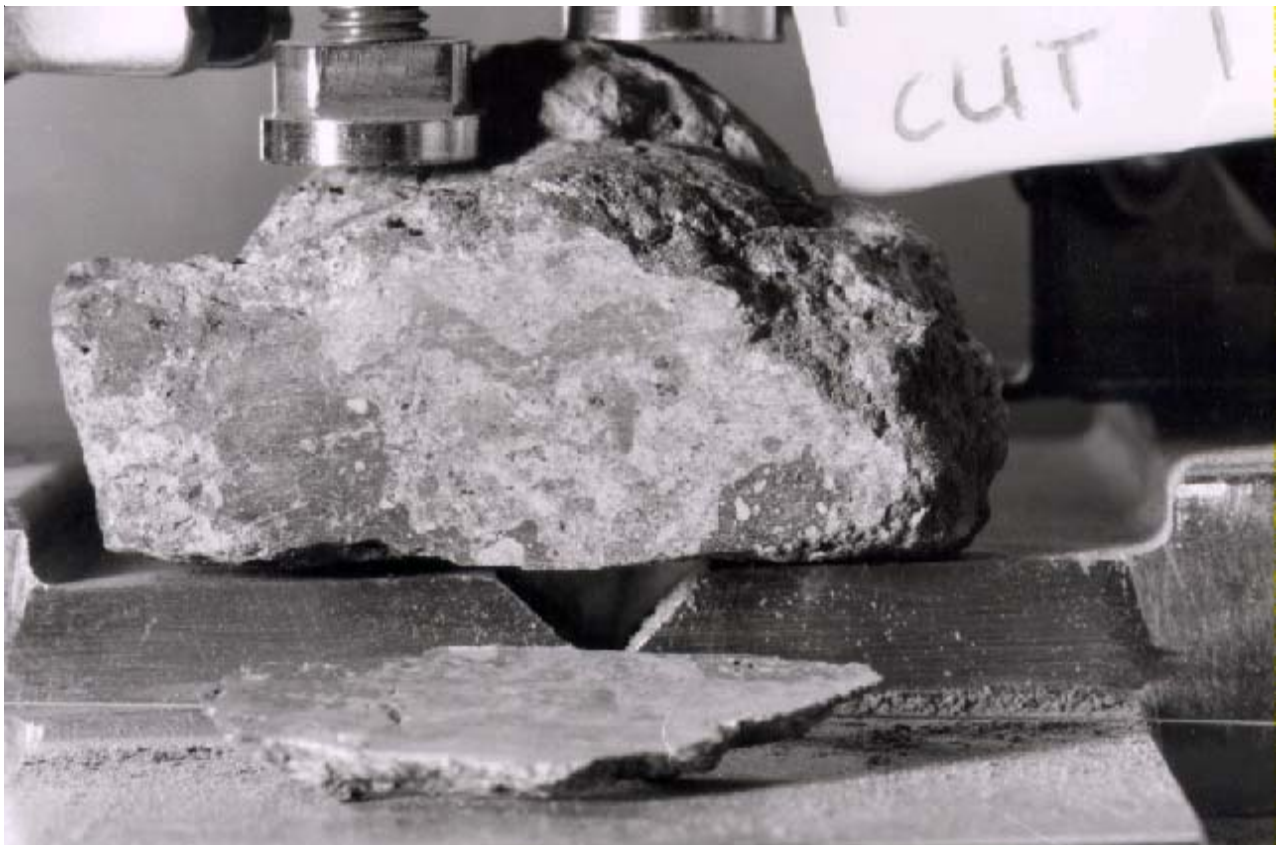
Figure 14: Photo after 1st saw cut of 12013. End piece ,8 is laying in the foreground. NASA# S70-40679
