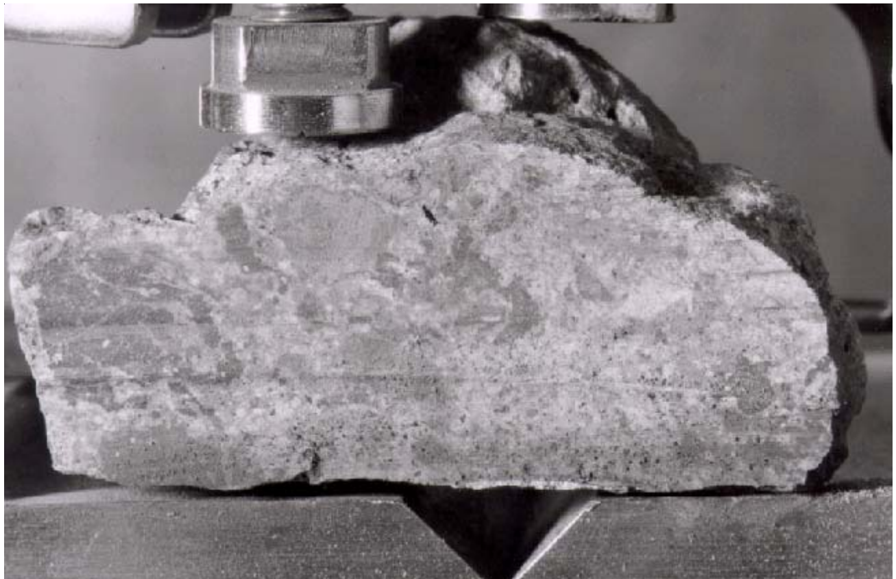
Figure 16: Photo after 3rd saw cut of 12013. NASA#S70-40682. Compare with figure 2.
