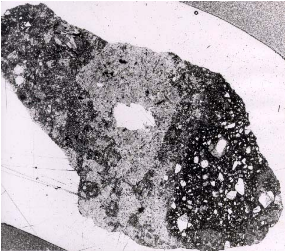
Figure 5: Photomicrograph of thin section 12013,6 showing "felsite" clast. Field of view is 11 mm. NASA # S70-25410.
