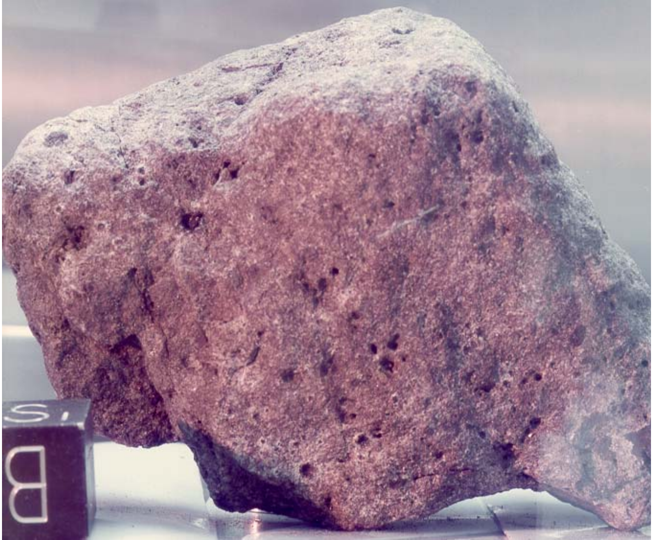
Figure 1: Photo of 12016,0 showing vesicles and zap pits on surface. Cube is 1 in. NASA# S75-33942.
