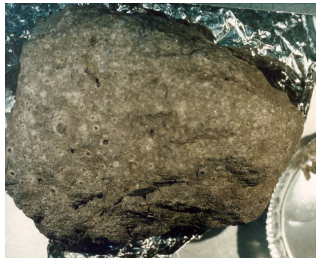
Figure 8: Pitted surface of 12019,0. NASA S91-38942. Sample is 8 cm across.
