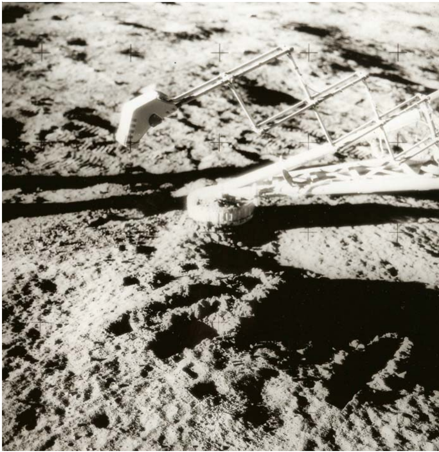
Figure 2: Photo of scoop on Surveyor III with trench dug in soil. AS12-48-7128.
