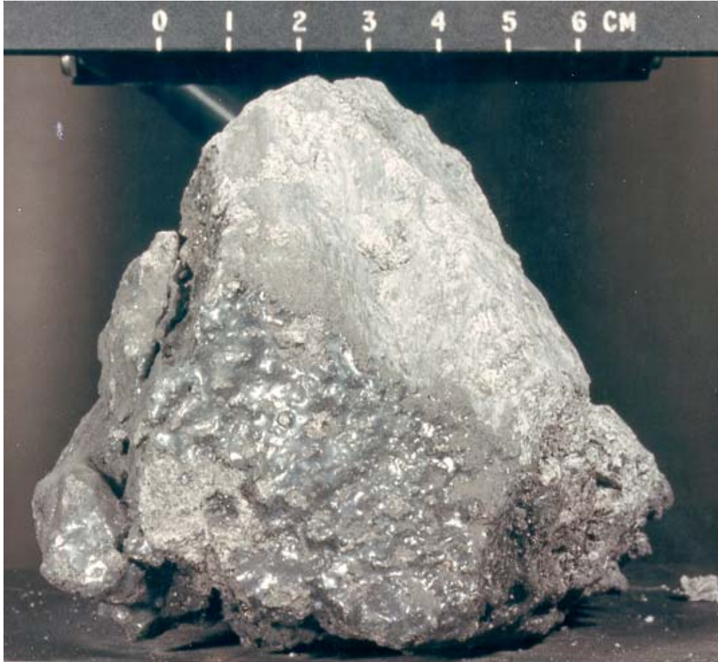
Figure 1: Photograph of 12054,0 showing shiny glass coating and large (cm-sized) glass-lined micrometeorite pit with surrounding spall zone. The light-colored area was below the soil line and protected from the glass splash. Scale is in cm. NASA photo # S69-62793.
