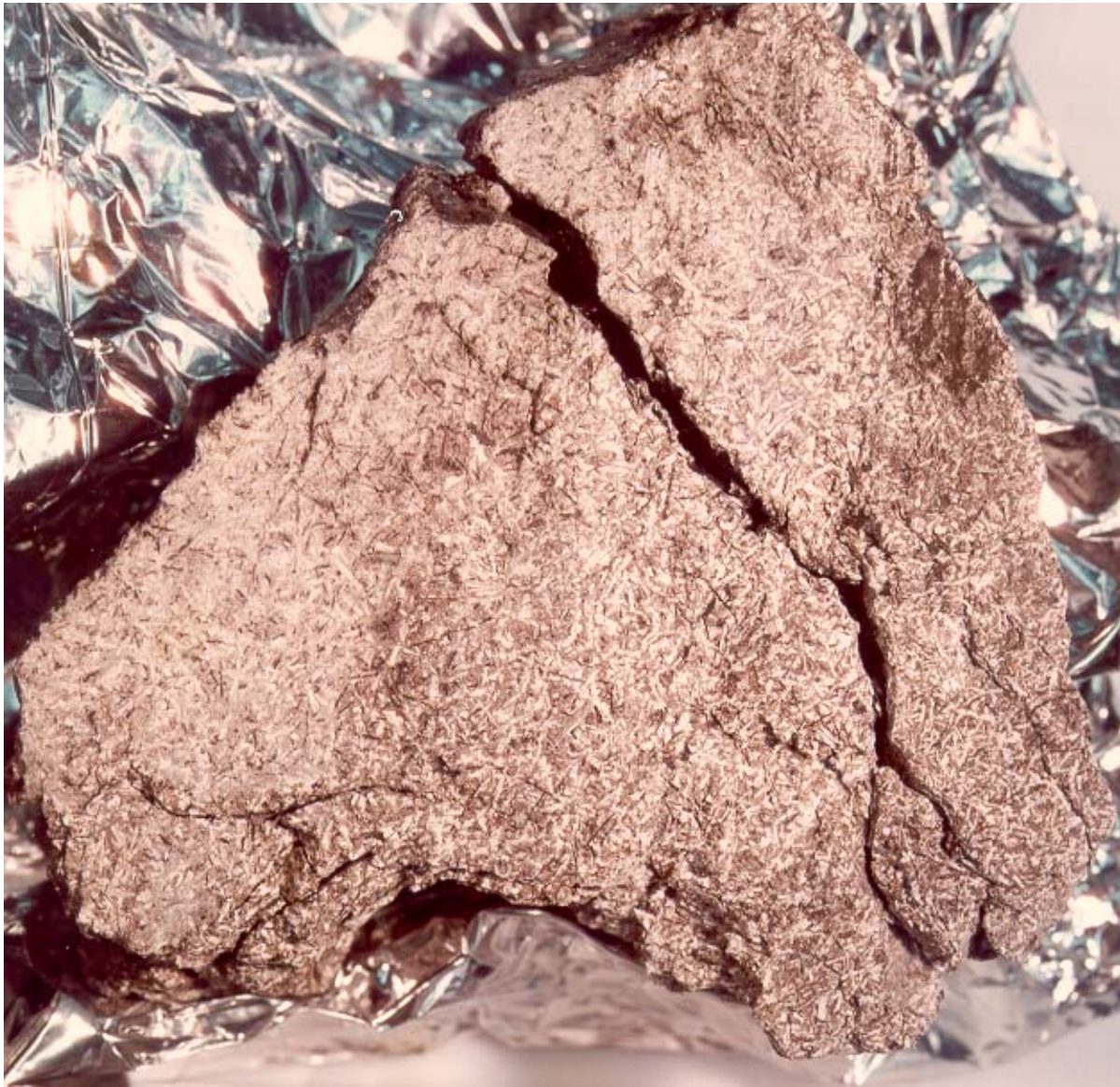
Figure 8: Photo of end-piece 12054,11, after sawing, illustrating basaltic texture. NASA # S75-34420. Sample is 7 cm across.
