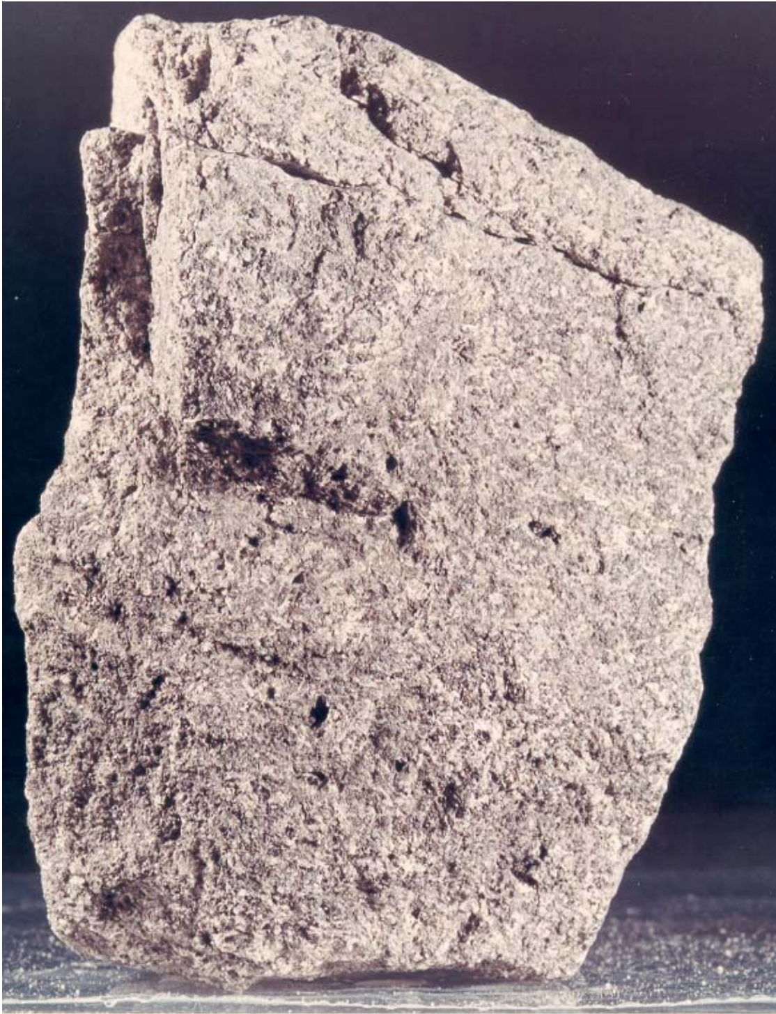
Figure 1: Lunar basalt 12064. Sample is 7 cm across. NASA # S70-44454.
