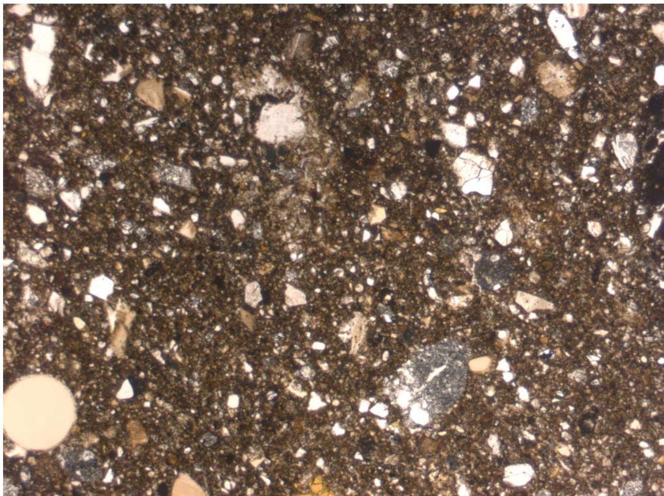
Figure 3: Thin section photomicrograph of 14042,26 showing glass bead (300 micron). Field of view is 2.8 mm. Photo by C Meyer.
