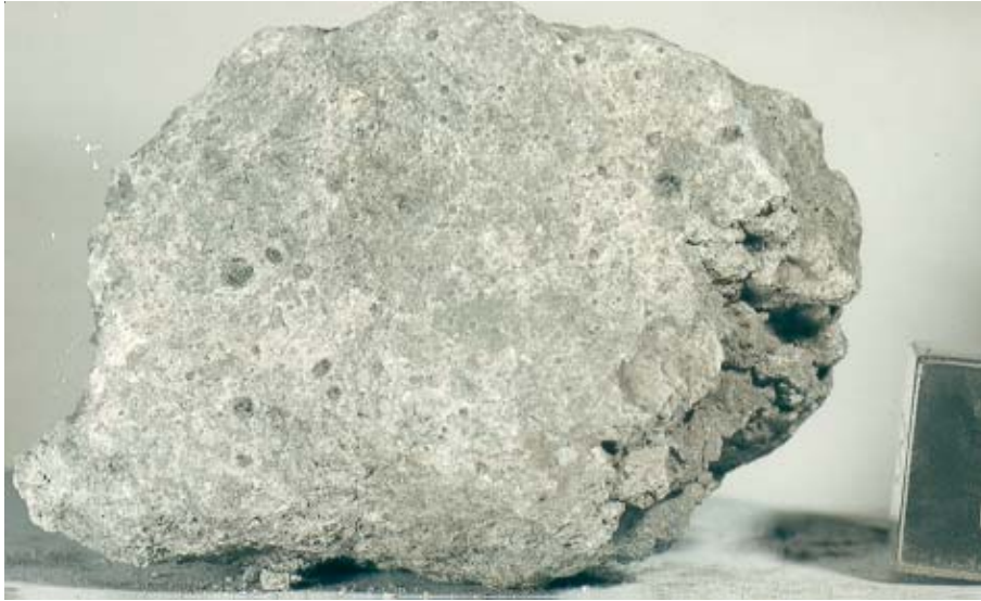
Figure 1: Photo of surface of 14066 showing zap pits. Cube is 1 inch. NASA S71-29233.
