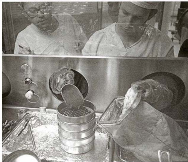
Figure 1b: Sieving soil sample in SNAP.
