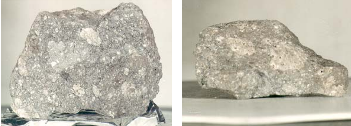
Figure 1: Bottom and side views of 14316 showing blueish internal color and clastic nature. Note also the zap pits on the top surface. Sample is about 2 inches long. NASA S71-29227 and 29232.
