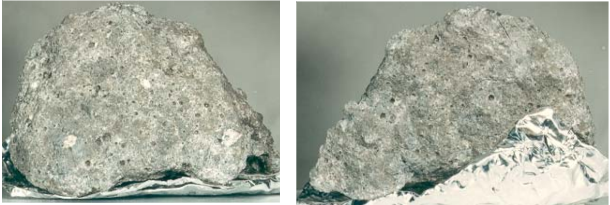
Figure 1: Two views of 14320 showing heavily cratered surfaces and white clasts. NASA S71-29196 and 29195. Sample is 6 cm across.
