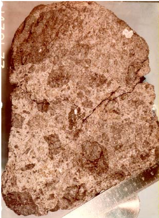
Figure 2: Photograph of initial saw cut through 14321. This is the west face of 14321,37. The white clast is W1 (c2). The scale is in cm. NASA photo S78-33119.
