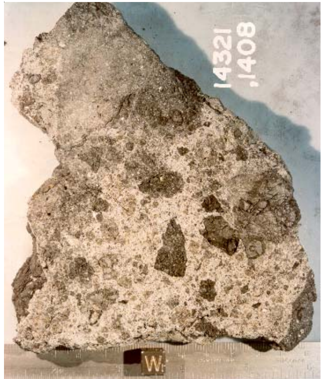
Figure 3: Photo of 14321,1408 illustrating light breccia matrix with dark aphanitic breccia clasts. Cube is 1 cm. Photo # S86-26402.
