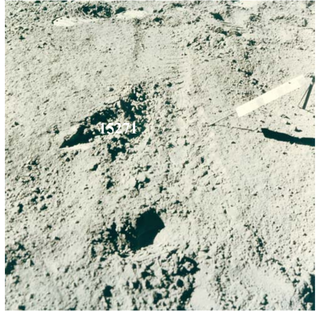
Figure 2: Picture of hole dug in rover track to obtain soil sample 15270. AS15-85-11657. Gnomon for scale.
