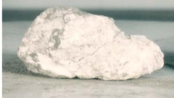
Figure 1: Photo of 15362. NASA S71-49627. Sample is about 2.5 cm long and 1 cm in cross section.
