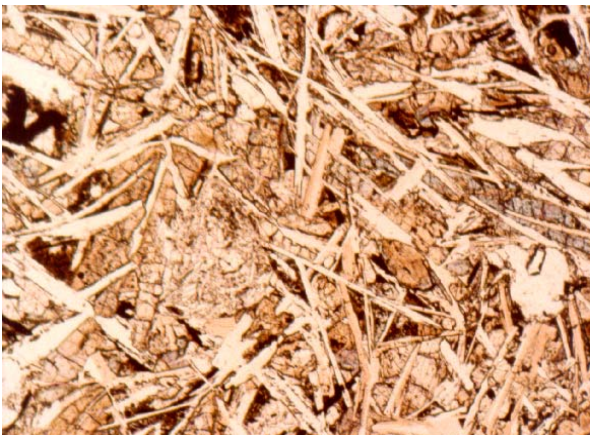
Figure 2: Photomicrograph of thin section of 15382 showing bent plagioclase crystals intergrown with pyroxene. NASA # S79-27741. Field of view is 2.7 mm. Photo is "off-color" because of fading of print.
