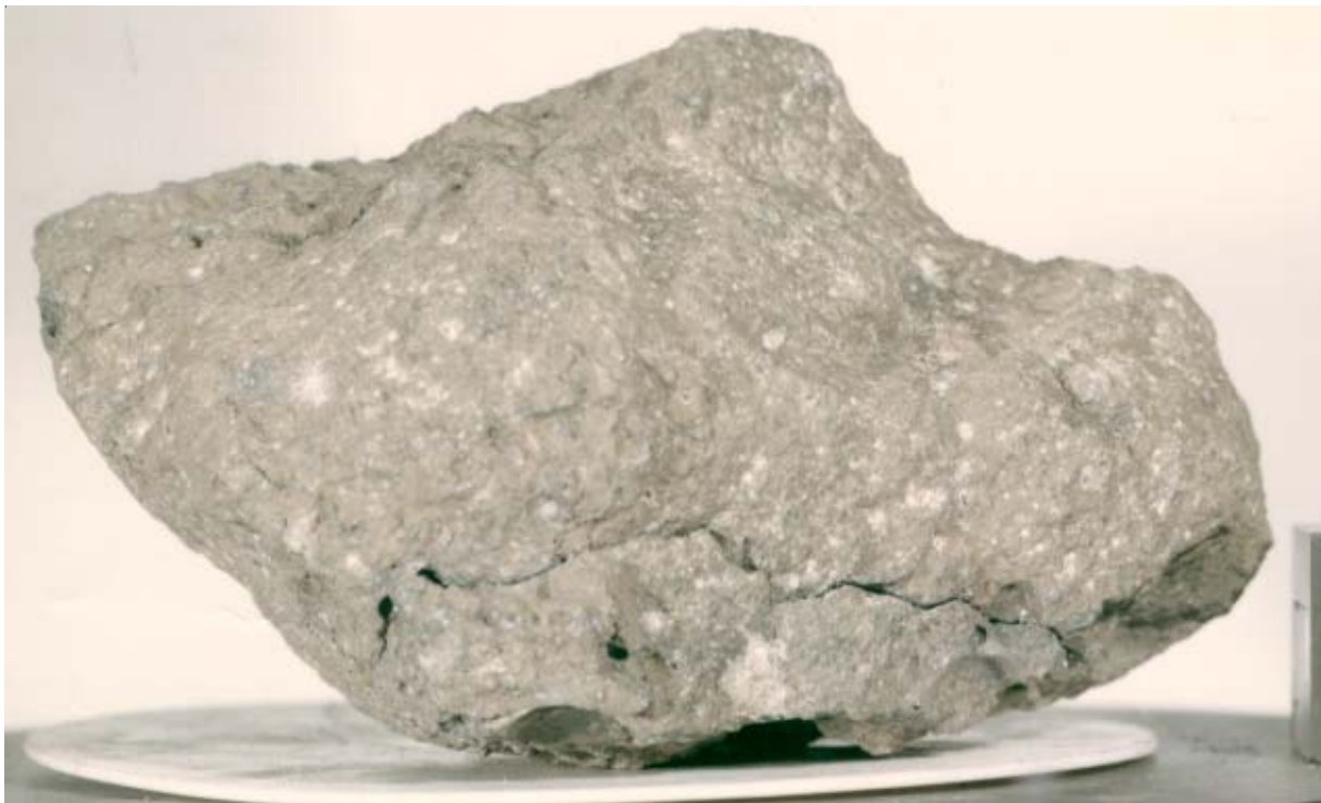
Figure 4: Original photo of 15418 showing a few zap pits and a penetrating fracture. Note the portion of a very large vesicle on the bottom. NASA S71-44865. Sample is 11 cm long.
