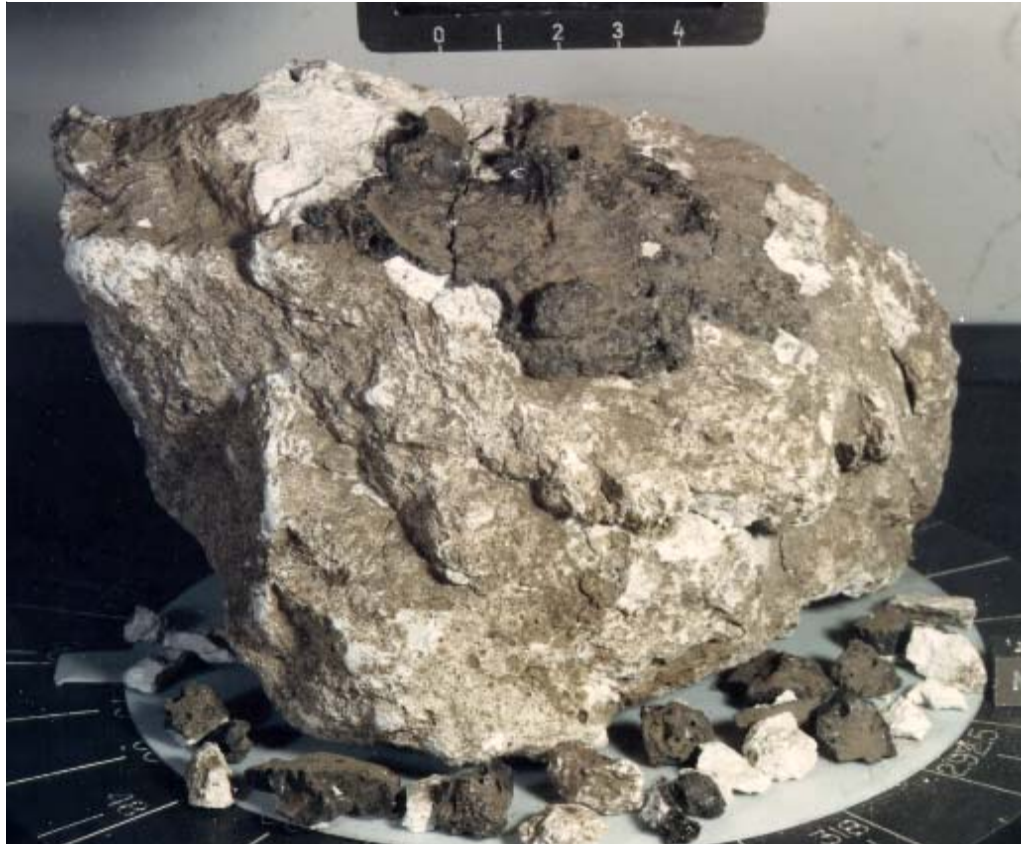
Figure 1: 60025. NASA #S72-41586. Cube and scale are 1 cm. Note the thick black glass coating and numerous micrometeorite pits.
