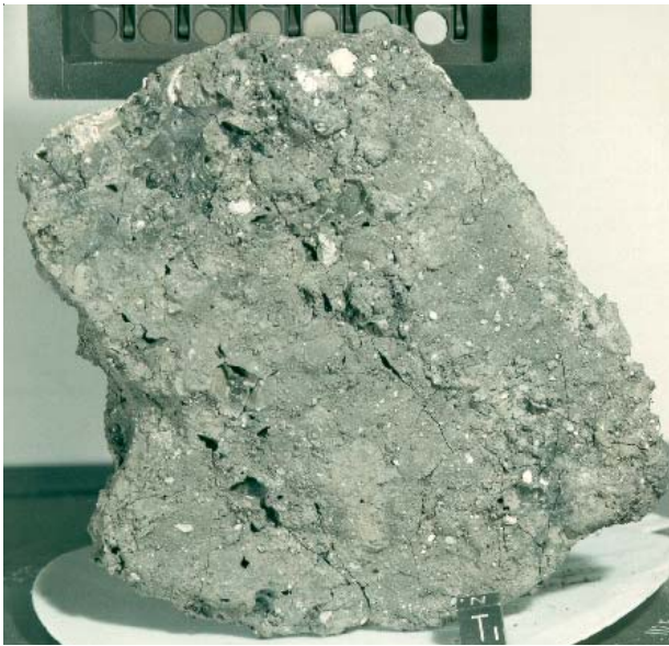
Figure 2: Bottom surface of 60035 showing attached black glass. NASA S72-38301. Cube is 1 cm.
