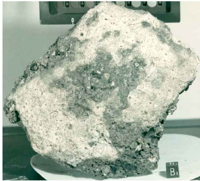
Figure 3: Top side of 60035 showing numerous zap pits. NASA #S72-38300. Cube is 1 cm.
