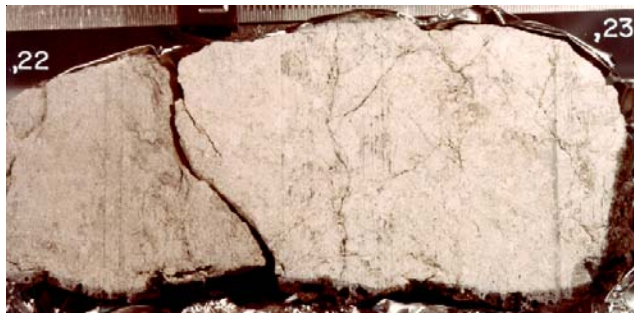
Figure 10: First saw cut, butt end ,22 and ,23 of 60035. NASA # S80-35176. Scale is in cm.
