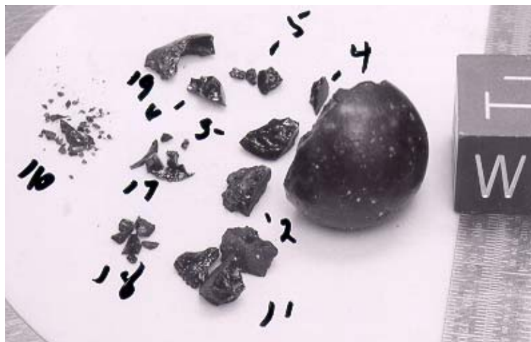
Figure 7: Numbering the splits of 60095. Splits ,1 and ,2 were from the large piece in figure 6. Other pieces broke off due to pressure of vise.
