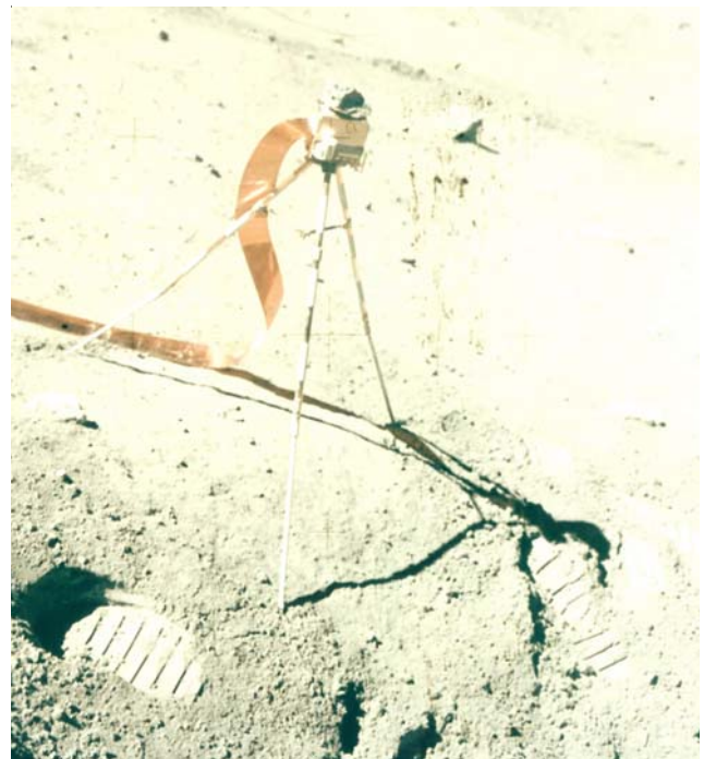
Figure 10: Photo of Lunar Portable Magnetometer with 60335 on top. AS16-116-18721.
