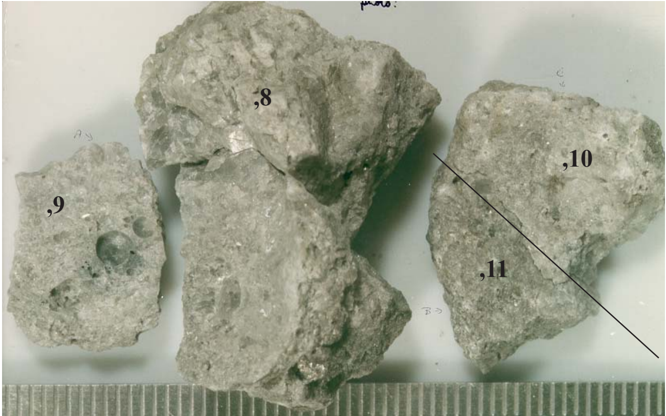
Figure 1: Photo of 60618. These three pieces fit together. Large round vesicles (4 mm) are prominent on the backside of center piece. Large pieces of plagioclase (anorthosite, 10) were surrounded by melt rock (,11). NASA S73-20462. Scale in mm.
